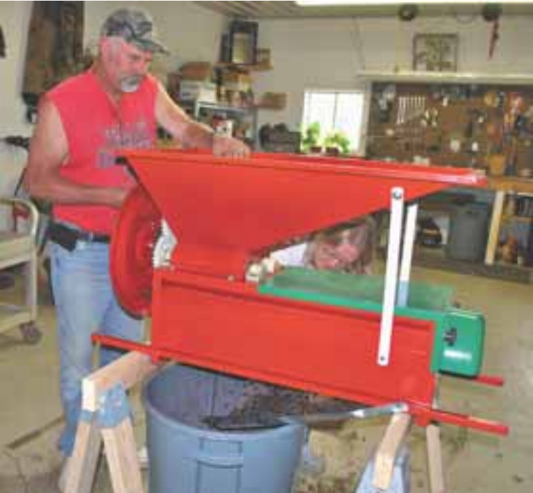
Russell and Karen work their grape destemmer-crusher machine. In 20 minutes, they can finish a job that previously took a room full of people four hours.
